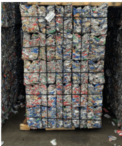
UBC – Briquette with Steel Bands
